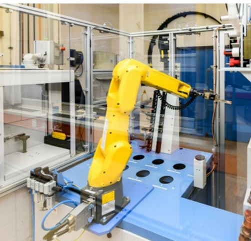
This robot analyzes stamping samples fully automatically.
